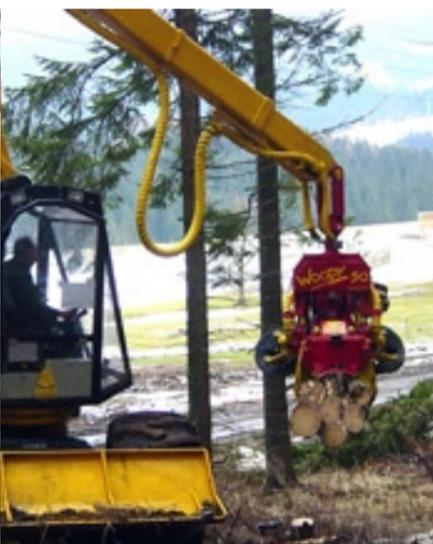
The upward folding feed unit provides a fully adequate loading claw with endless rotation. => It is possible to pick up side by side lying logs.
