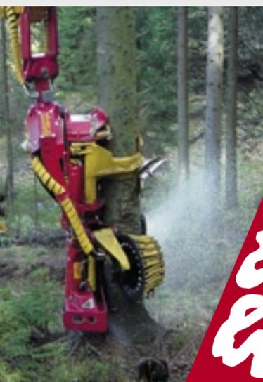
The relatively extensive face-to-face length allows for controlled felling of large trees.
