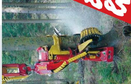
The big overall length of the WOODY allows a controlled felling of large trees.
